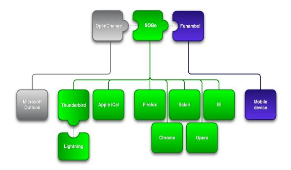
Standard protocols such as CalDAV, CardDAV, GroupDAV, HTTP, IMAP and SMTP are used to communicate with the SOGo platform or its sub-components. Mobile devices supporting the SyncML standard use the Funambol middleware to synchronize information.
